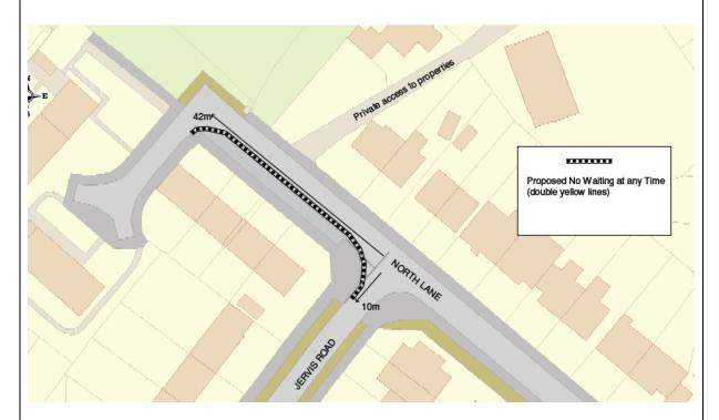
Restrictions were proposed on the south west side of the carriageway to remove the "chicanes" caused by parked cars and enable vehicle access. Removing parking on one side should remove the necessity of vehicles parking on the footway to enable others to pass. Restrictions on the west side ensures houses opposite can access and leave drives opposite. Some parking amenity remains on the east side of the carriageway between the residential drive access points.
