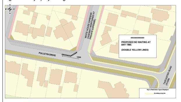
The proposal (15m from the projected western kerbline of White House Gardens west for 15 metres) was designed to prevent parking close to the junction causing the reported issues with access and sight lines on exit.
